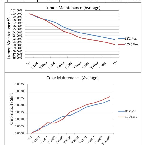
Observation of LED light sources failures, including the failure conditions and time of failure: No failure observed
