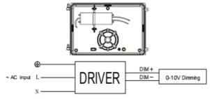
**3.** Please connect all cables and terminals according to the wiring diagram. Please pay attention to the grounding.
