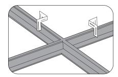
⑤ Check the clips well fasten to T-BARM (Main/Cross ceiling tee.)
