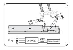
Please connect all cables with connectors one by one according to the wiring diagram. Please note that the wires passing through the entry holes need protective jackets, and pay attention to grounding.
