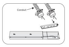
® Insert the cable into driver box.
