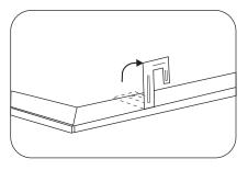
② Lift the mounting clip on the edge of panel.
