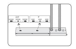
Adjust the toggle switch, and customers can choose the wattage and color temperature of lamps on site according to their own needs.
